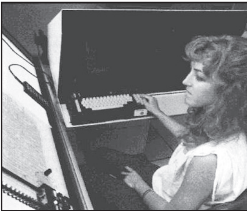
Photo 4: Digitizing. Computer aided design (CAD) technician Lisa F. enters a cell layout into the data base. The cursor on the light table is used to transfer precision measurements to the computers. An already digitized cell is shown on the video display.
