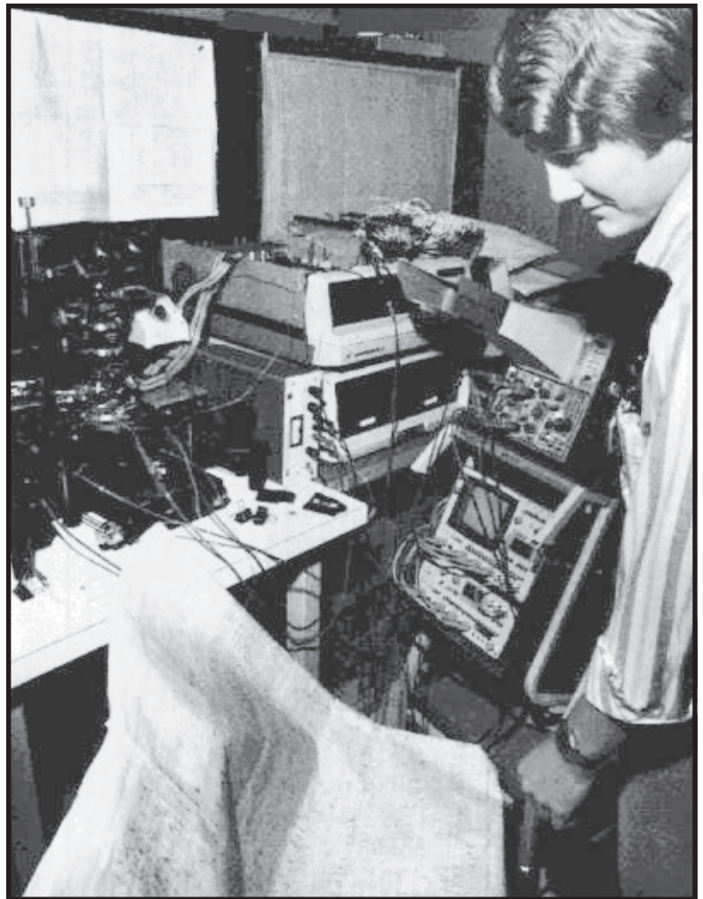
Photo 5: First silicon engineering analysis. Logic and circuit design engineer Bob Thompson tracks down a weak node in the first batch of 6801 chips. The 6801 die is packaged, but not sealed, so that internal nodes may be probed while in operation. Viewing through a microscope, a probe can be placed at critical points equivalent to the layout plot. The chip itself is running a modifies EXORcisor system, and the scope actually displayed an internal signal with excessively slow rise time.
